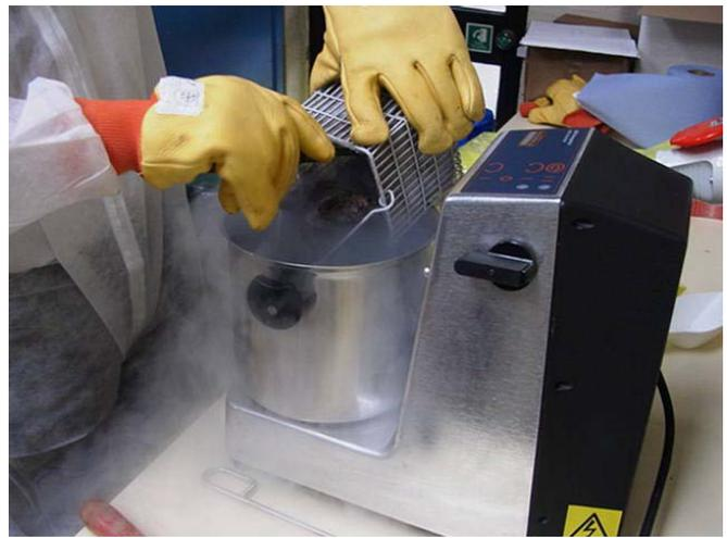
d) Transferring the sample to the homogeniser
